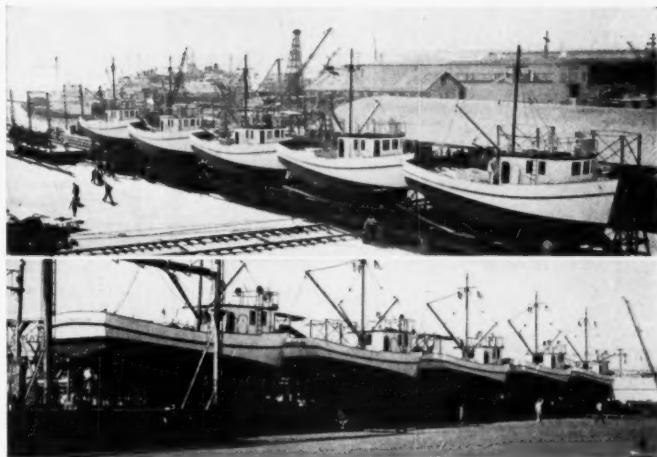
Fleet of five 54-foot welded-steel shrimp trawlers as they were readied for launching in October at the San Diego plant of National Steel and Shipbuilding Corporation. The vessels are shown here on the 340-foot extension of one of National Steel's marine railways. The trawlers carry Atlas diesels, driving through Monel shafts.
